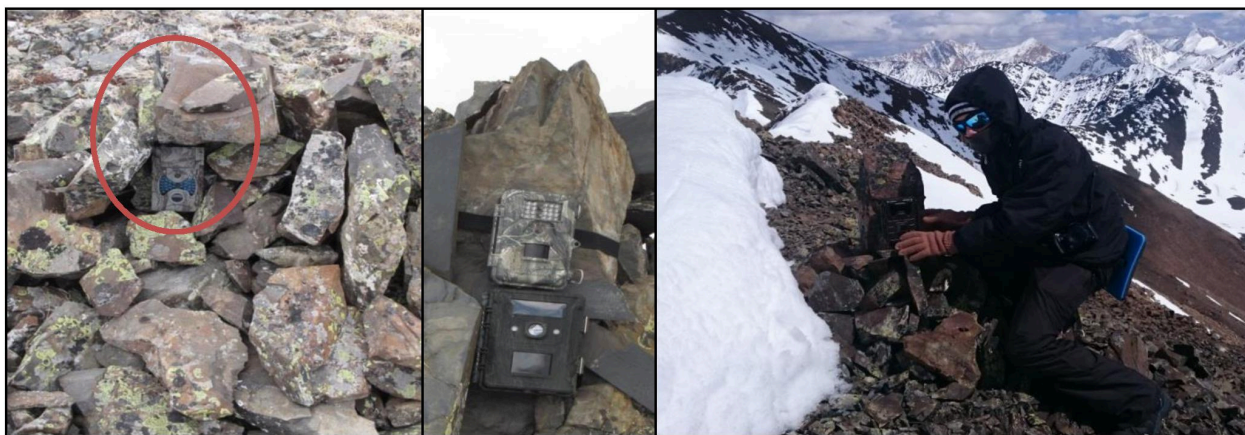
Figure 4. Different models of camera-traps have been used: Boskon Guard with MMS function (with antenna) hidden in a rock cairn (left) ; Bushnell and Bestok camera-traps (middle) ; installation of a Bushnell trap by Audrey Jost (the author) (right)
